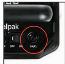
The fuse in the Travelpak control panel is located on top of the control panel as shown. To replace, simply unscrew the fitting. Always replace the fuse with the same rating.
